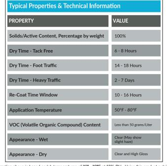
Information above is based on lab temperatures of 70° - 72°F at 50% RH. Using this product outside these conditions may affect the accuracy of the information above. Always test prior to use!
