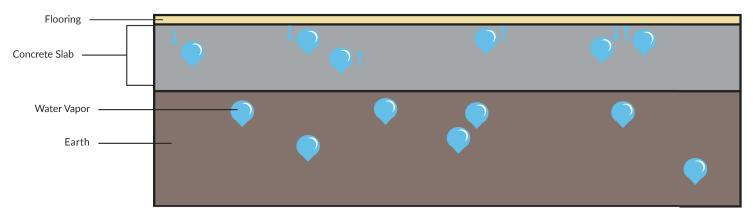
M.V.B 100 is a high-performance epoxy primer system designed to reduce water vapor transmission. When applied to a properly prepped concrete, M.V.B 100 has shown to have improved adhesion to concrete surfaces where moisture is an issue and other high-performance coatings have failed.
